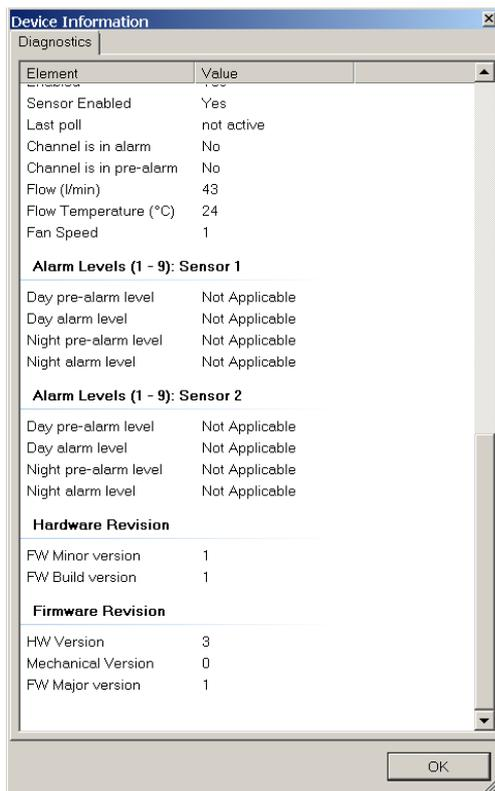
**NOTE:** To run the upgrade tool, PipelQ must be installed on the PC. But the PipelQ application should not be in the 'connected' software state with the FAAST LT device, because it will then be occupying the PC COM port required by the upgrade tool.
