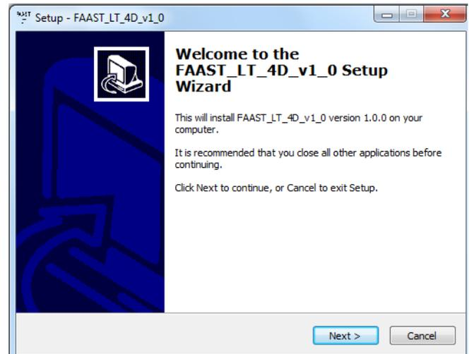
The setup wizard will first install a proprietary Renesas Flash Development Tool, required to re-write the microcontroller memory, and then it will run the upgrade routine itself.
