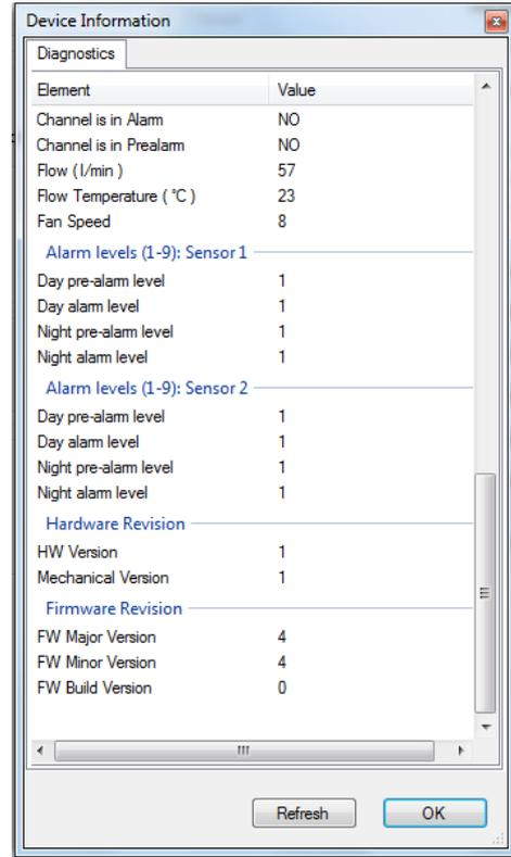
It is recommended that the firmware revision to Minor Version **4Dv1** is noted indelibly on the label provided and mounted beside the nameplate label on the inside of the unit's door.
