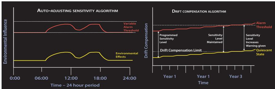
The unique auto-adjusting sensitivity algorithm automatically adjusts the alarm threshold to compensate for short-term changes in the environment which could otherwise result in unwanted alarms. Two alternative auto-adjusting sensitivity settings are available. These adjustments do not compromise the detector's ability to respond quickly to a fire incident.
