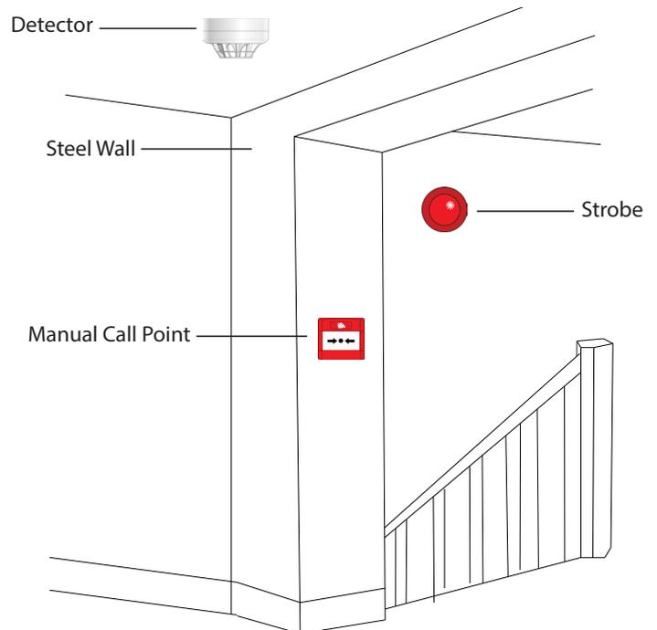
In this arrangement the sounder-strobe could have been located on the wall opposite to the manual call point at a required height.
