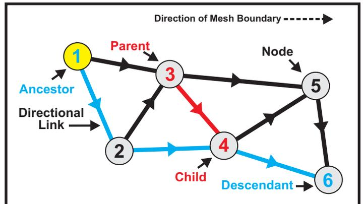
Note the unique and important Back-up Node #2; this has only one parent – the gateway. Its importance in the network is described below.
