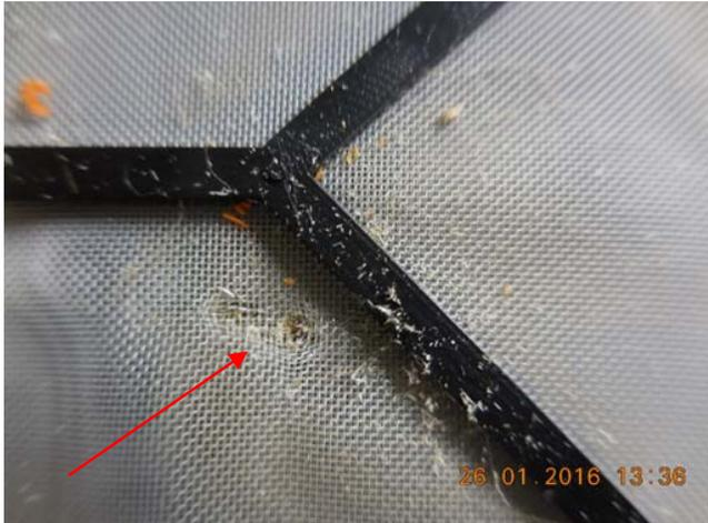
This unit gave a fault because of a spider's web inside. It is recommended that the inlet and outlet connections remain plugged prior to use and during installation. And the outlet should be temporarily sealed if the device is turned off during maintenance periods.
