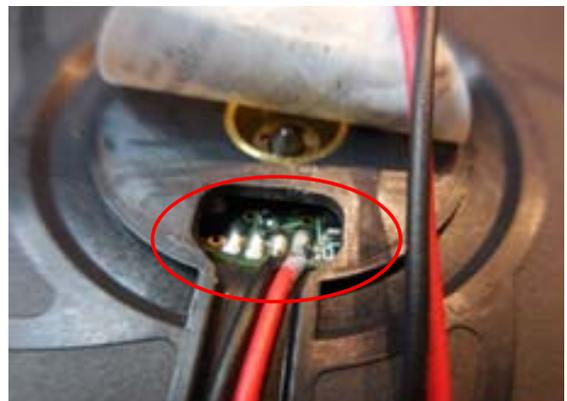
Examples of internal parts coated by oil from the environment or from the use of unsuitable paraffin-based test smoke:
