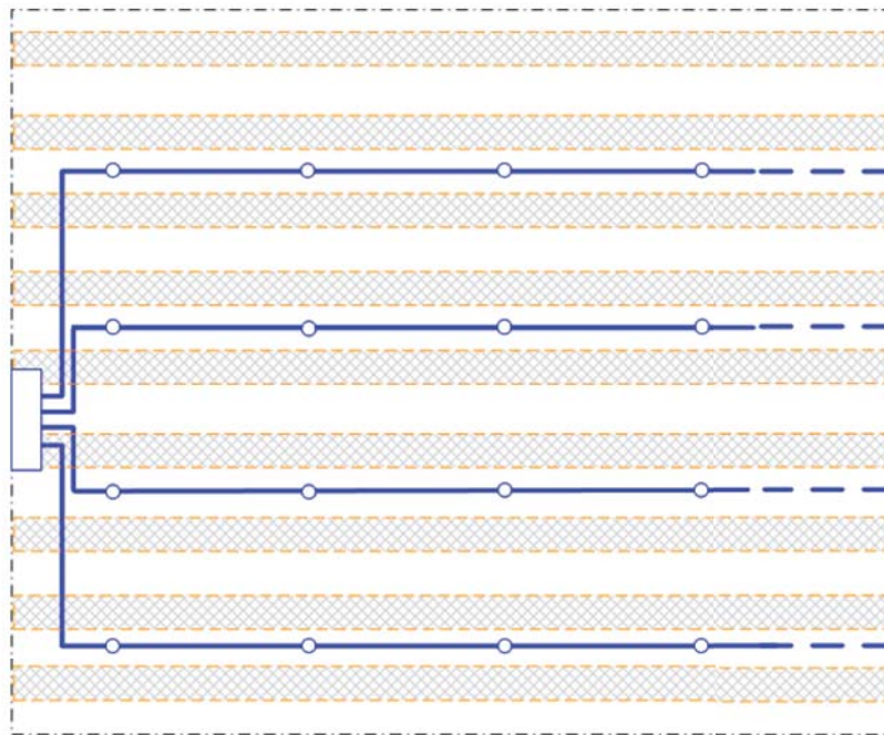
Figure 3 – Storage rack area ceiling System Sensor sampling Pipe Layout (Non-Branched, pipes parallel to rack orientation).
