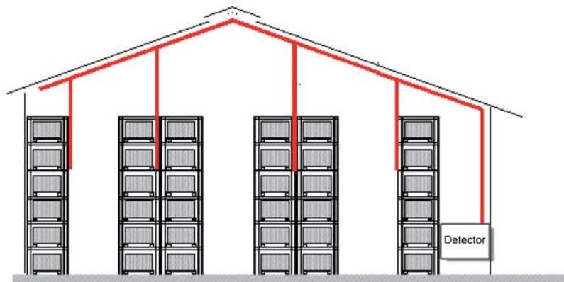
Figure 8 – Example of drop-down pipes for In-rack Detection.
